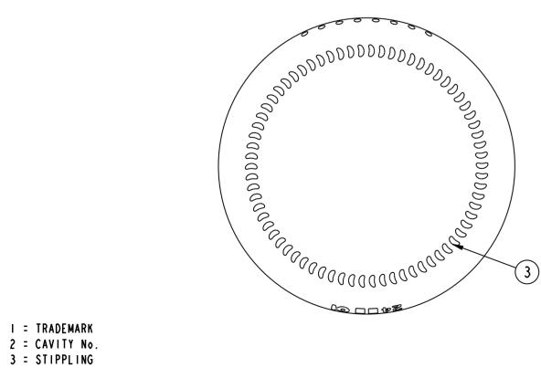
2 = CAVITY No. 3 = STIPPLING THE SHAPE OF STIPPLES IS ONLY AN INDICATION AND THE CONSTRUCTION IS AT THE PRODUCTION PLANT DISCRETION. 4 = CAVITY CODE
